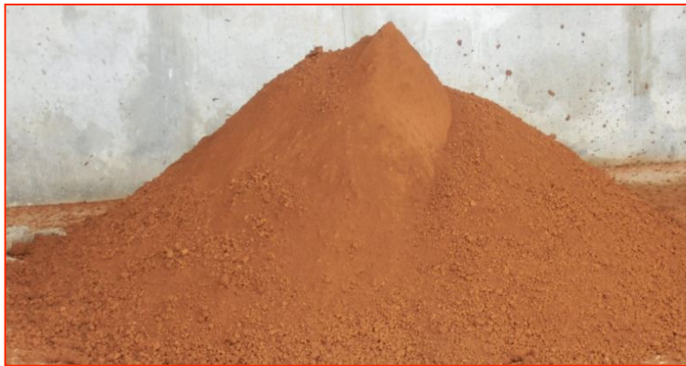
Figure 2: A heap of dry and flowable DBR after discharge from the HiBar disc filter plant
