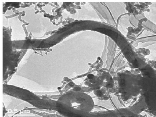
Figure 4: TEM image illustrating carbon nanotubes formed from butane cracking at 800 °C as presented in reference 2 and reproduced with kind permission from Elsevier Taking advantage of their magnetic nature for facilitated separation, the composites have been applied to the treatment of model water samples.
