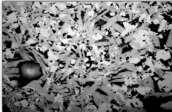
Figure 4: Microstructure of sinter with 5 % LABR. Residual grains of magnetite– white, ferrite – grey, glass phase – dark grey. Reflected light, magnification \times 500
