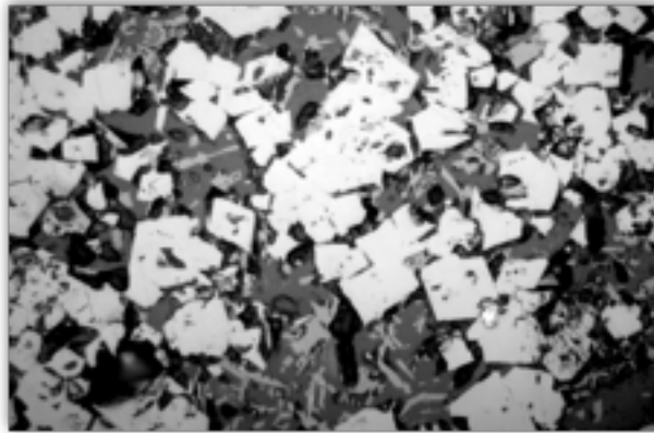
Figure 2: Microstructure of sinter with 1 % LABR. Glass phase – grey, needle crystals of ferrite – light grey. Reflected light, magnification \times 500
